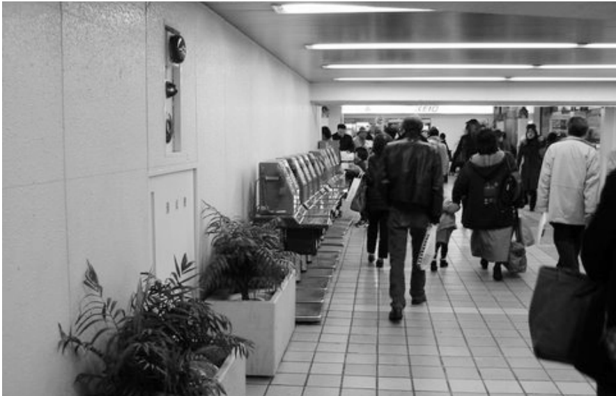
Fig. 2-22 An alarm bell on the walls of a pedestrian walkway at a railway station is also carefully prevented from undesirable use by lining them with plant pots.
